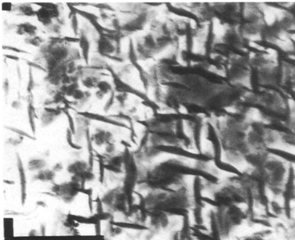
Figure 5 Micrograph and electron diffraction pattern of the Fe-20Mo alloy aged at 550 °C for 100 h, showing plate-like particles of the Fe 2 Mo phase, and the additional system of Fe 2 Mo phase reflections.
